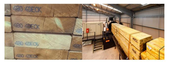
At Södra Wood we stock imported European Redwood KD C24 strength graded deck joists that have been high pressure treated to UC4 for use in external and ground contact applications, such as decking framework.
