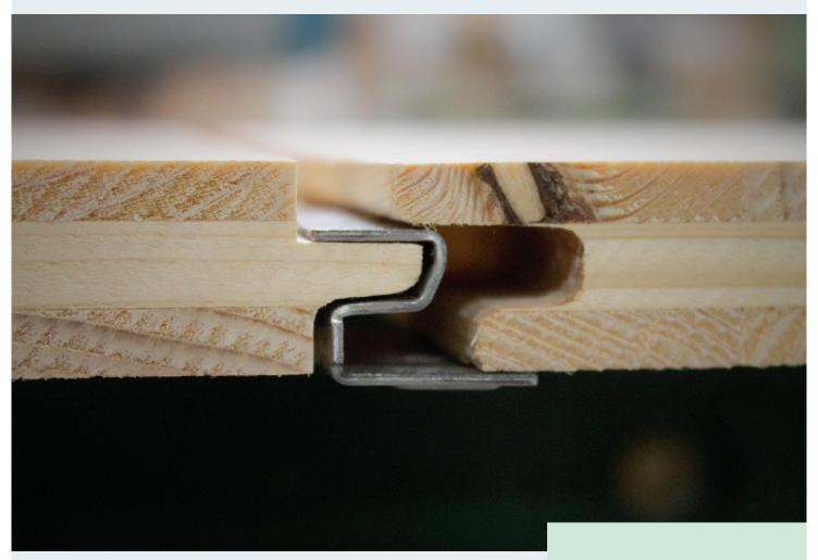
Hidden clips allow us to install cladding without nails or screws. This means that the surface of the cladding can be kept clean and tidy without making any holes. It also means that the panels chosen can be fully coated before they are installed, which enables higher quality and saves time.
