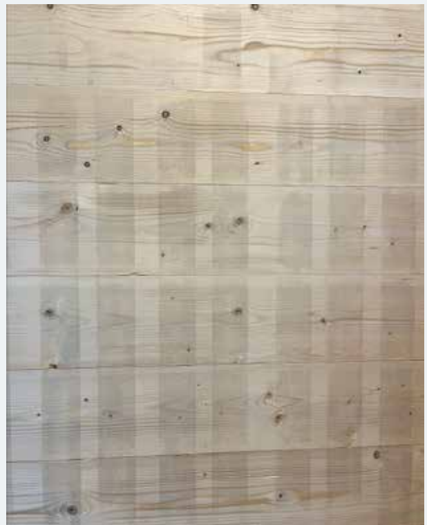
Example of a 'non-visible surface quality' where pressure marks may occur.
