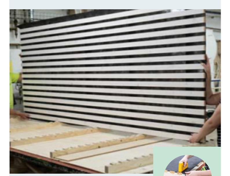
Södra's cassettes are elements of wooden slats that are assembled to create a system solution, designed to save time and space in the workplace. The cassettes contribute to efficient and simple installation, while also giving a clean and attractive impression.
